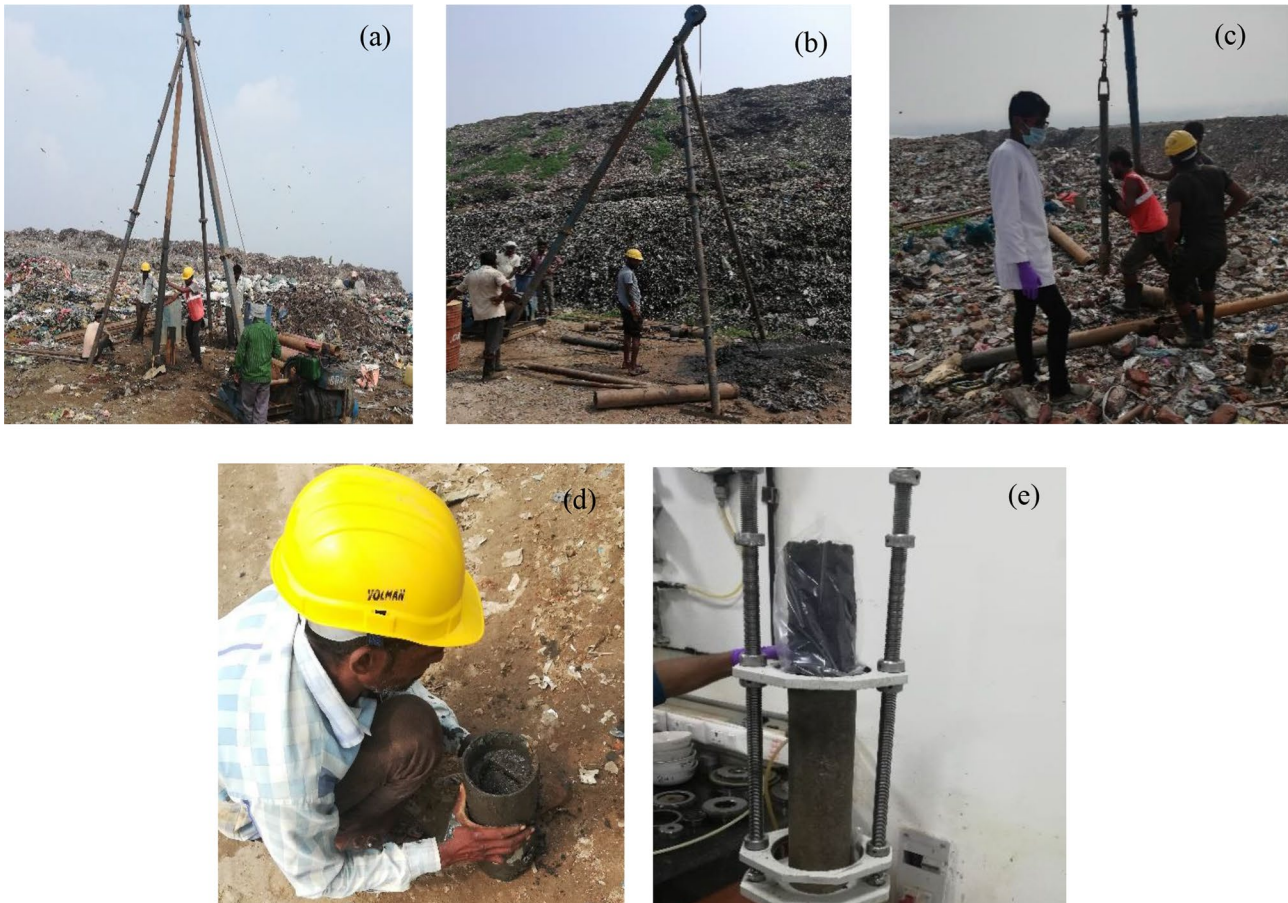
Fig. 1 Sampling through drilling, a Drilling from the top level of dumpsite, b drilling from the mid-height of dumpsite, c bailer operation at 20 m depth from the top of the dumpsite, d sample in sampling tube retrieved from boreholes, e sample extrusion in the laboratory
